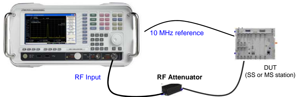
Fig. 1 CDMA2000 measurement setup
