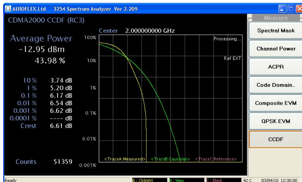
Fig. 10 Result of measuring CCDF for CDMA2000 signal
